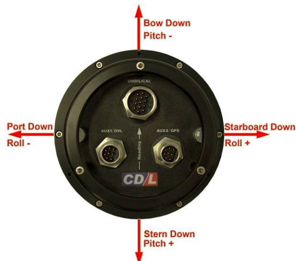
Figure 5.1: Pitch and roll convention (MiniRLG,EM3000)
