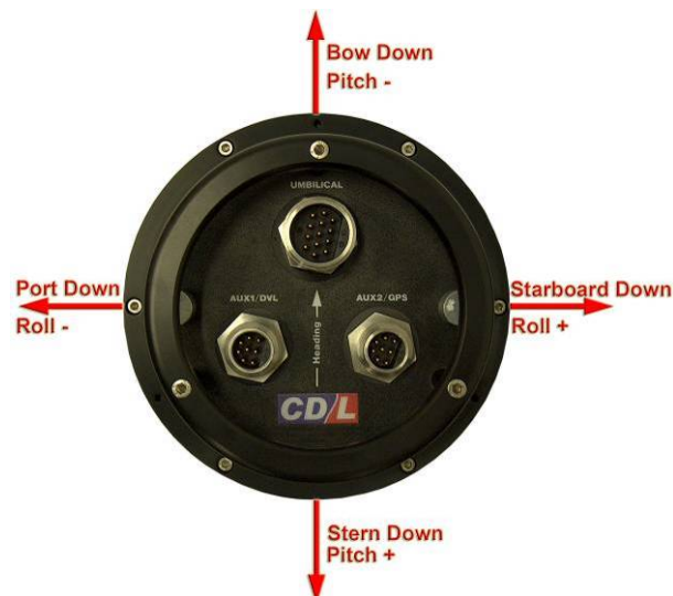
Figure 5.1: Pitch and roll convention (MiniRLG)
